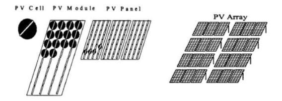
Figure 4: Elements of SPV system
