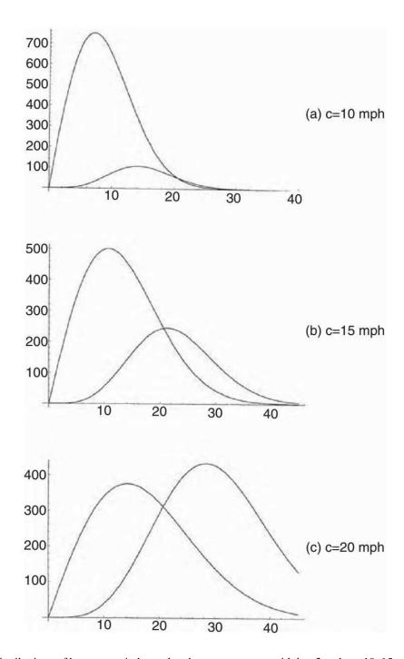
Rayleigh distributions of hours vs. wind speed and energy per year with k=2 and  $c=10,\,15,\,$  and 20 mph.
