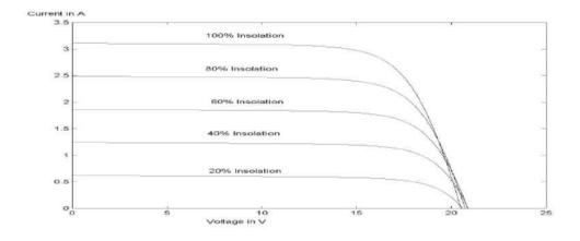
Figure 6: I-V characteristics for different insolation levels
