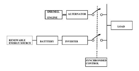
Figure :Parallel configuration
