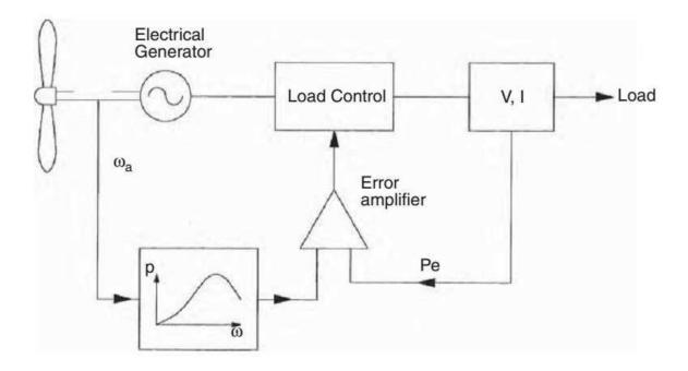
Maximum power operation using power control scheme.
