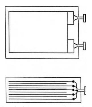
Electrochemical energy storage cell construction.
