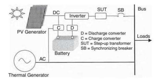
Electrical schematic of the grid-connected PV system
