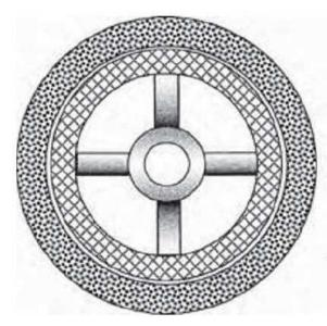
Rotor of two-composite fiber rim for high specific energy and safety
