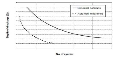
Figure 8: No. of battery cycles and Depth of discharge
