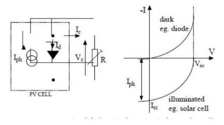
Figure 2: Equivalent circuit of a solar cell
