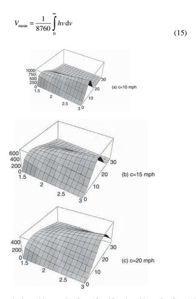
Three-dimensional h-v-k plots with c ranging from 10 to 20 mph and k ranging from 1.5 to 3.0.
