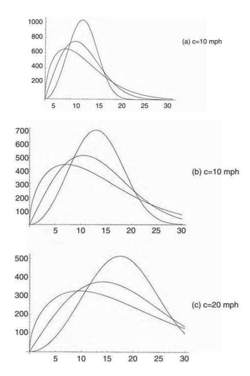
Weibull distributions of hours per year with three different shape parameters  $k=1.5,\,2,$  and 3, each with scale parameters  $c=10,\,15,$  and 20 mph.
