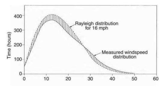
Rayleigh distribution of hours per year compared with measured wind speed distribution at St. Annes Head, Pembrokeshire, U.K.
