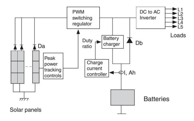
Peak-power-tracking PV power system showing major components
