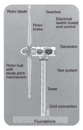
Horizontal-axis wind turbine showing major components.
