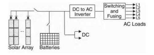
PV stand-alone power system with battery.
