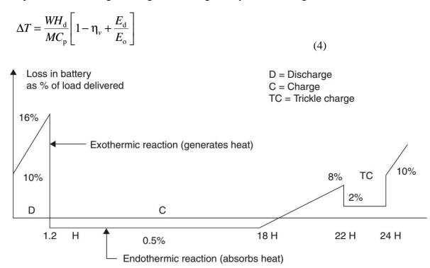
Internal energy loss in battery during C/D cycle showing endothermic and exothermic periods.
