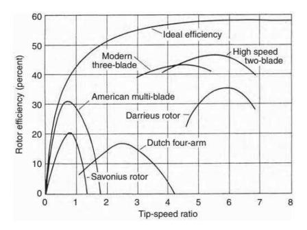
Rotor efficiency vs. V<sub>o</sub>/V ratio for rotors with different numbers of blades.
