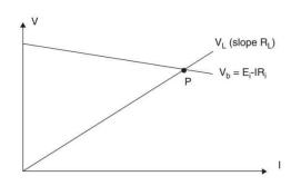
Battery source line intersecting with load line at the operating point.
