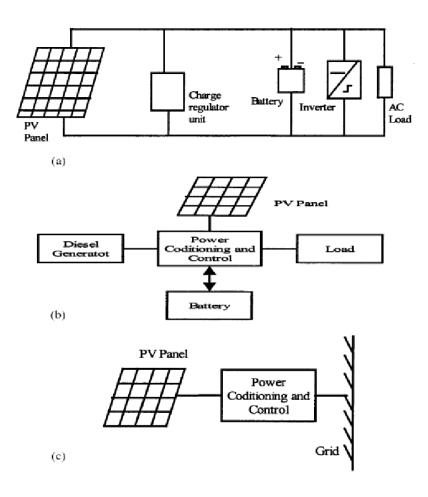
Figure 7: (a) Stand Alone PV system (b) PV-diesel hybrid system (c) Grid-connected PV system
