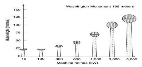
Tower heights of various capacity wind turbines.
