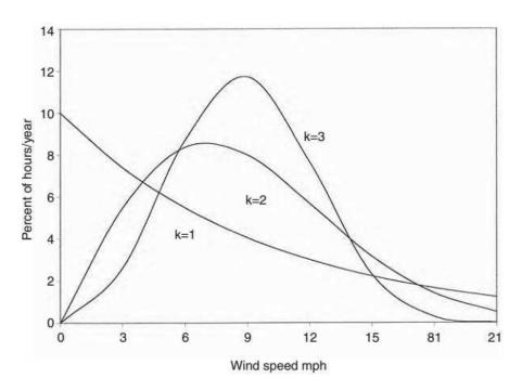
Weibull probability distribution function with scale parameter c = 10 and shape parameters k = 1, 2, and 3.
