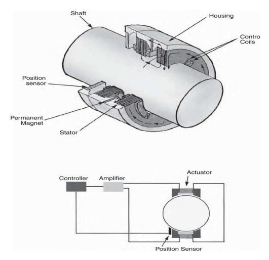
Avcon's patented homopolar permanent-magnet active bearing.
