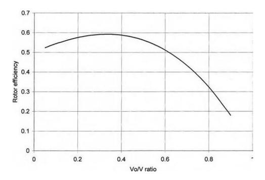
Rotor efficiency vs. V<sub>o</sub>/V ratio has a single maximum.
