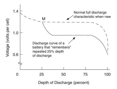
Memory effect degrades discharge voltage in Ni-Cd cell.
