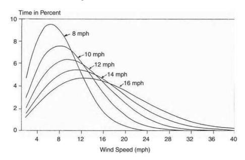
Weibull probability distribution with shape parameter k=2 and scale parameters ranging from 8 to 16 mph.
